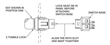
NOTE: Switch installation is permanent. Switch cannot be removed from lock after assembly. Attempts to separate switch and lock may damage switch.
